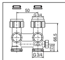
ZBU preset isolating fitting for filling and draining
