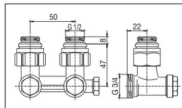
ZBU/CEW angle pattern preset isolating fitting for filling and draining
