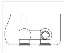
For radiators with integrated distributor G 1/2 female thread
