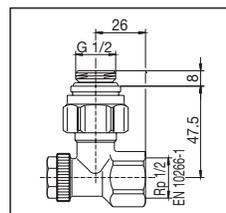
Angle pattern isolating fitting "Combi 3"<sup>\*\*\*</sup>
