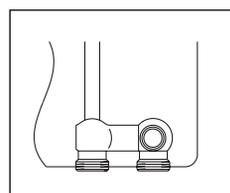
For radiators with integrated distributor G 3/4 male thread according to DIN EN 16313 (cone "Euro")
