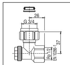
Angle pattern isolating fitting "Combi 3"<sup>\*\*\*</sup>
