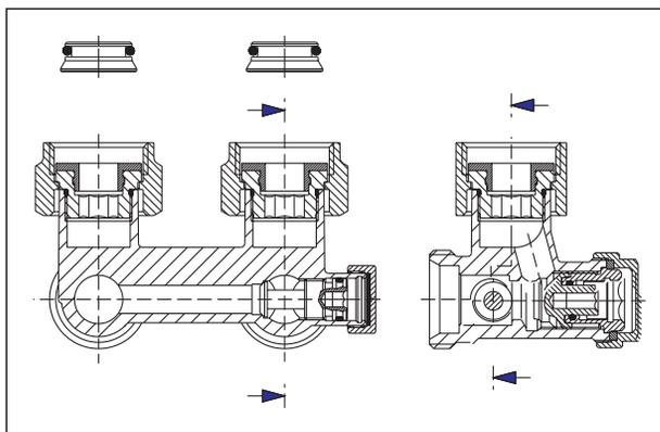
ZBU angle pattern preset isolating fitting for filling and draining
