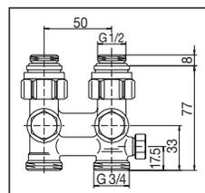
ZBU/CEW preset isolating fitting for filling and draining
