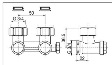
ZBU angle pattern preset isolating fitting for filling and draining
