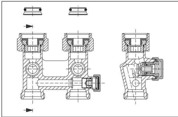
ZBU preset isolating fitting for filling and draining
