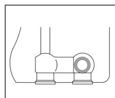
For radiators with integrated distributor G 1/2 female thread
